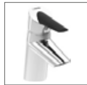
HANSAFIT one-hole single-lever basin mixer, DN 15 6509 2203 chrome incl. push-pop-up waste, connection with flexible pressure hoses projection: 98 mm
