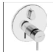
HANSASTELA trim kit with function unit single-lever bath mixer with vacuum breaker suitable for HANSABLUEBOX concealed unit* 8784 3041 chrome rosette without screws, round rosette, Ø 170 mm, function unit with BLUESWITCH diverter
