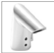
HANSAFIT electronic basin faucet, DN 15 mains supply 6541 2000 chrome sensory operation (infrared), without pop-up waste, incl. power supply and connection cable, flexible hoses projection: 85 mm
