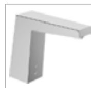
HANSALOFT electronic basin faucet, DN 15 battery-operated 5749 2211 chrome sensory operation (infrared), push-pop-up waste projection: 143 mm
