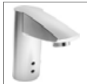
HANSAELECTRA electronic basin faucet, DN 15 battery-operated 6491 2211 chrome sensory operation (infrared), without pop-up waste, hygienic flush after 72 h for 30 sec at factory preset projection: 115 mm
