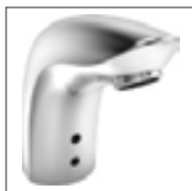
HANSAELECTRA electronic basin faucet, DN 15 battery-operated 6440 2211 chrome sensory operation (infrared), for cold or pre-tempered water only, without pop-up waste, hygienic flush after 72 h for 30 sec at factory preset projection: 96 mm
