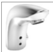
HANSAELECTRA electronic basin faucet, DN 15 mains supply 6441 2001 chrome sensory operation (infrared), incl. power supply and connection cable, without pop-up waste, hygienic flush after 72 h for 30 sec at factory preset projection: 96 mm
