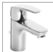
HANSA PINTO one-hole single-lever basin mixer, DN 15 4504 2283 chrome pop-up waste (metal), connection with flexible pressure hoses, HANSA 3S-Installation projection: 107 mm
