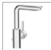
HANSAVANTIS STYLE one-hole single-lever basin mixer, DN 15 5254 2287 chrome pin operating lever (metal), connection with flexible pressure hoses, pop-up waste (metal) projection: 139 mm
