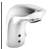
HANSAELECTRA electronic basin faucet, DN 15 mains supply 6441 2000 chrome sensory operation (infrared), incl. power supply and connection cable, without pop-up waste projection: 96 mm
