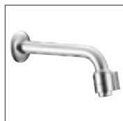
HANSANOVA wall-mounted basin valve, DN 15 0096 8101 chrome for cold or pre-tempered water only, can be shortened from 186 to 126 mm projection: 186 mm
