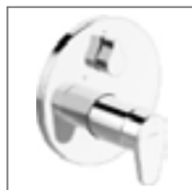
HANSASIGNATUR trim kit with function unit single-lever bath mixer with vacuum breaker suitable for HANSABLUEBOX concealed unit* 8063 3003 chrome rosette without screws, squared rosette, 150 x 150mm, function unit with BLUESWITCH diverter
