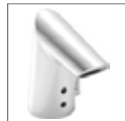
HANSAFIT electronic basin faucet, DN 15 battery-operated 6541 2210 chrome sensory operation (infrared), without pop-up waste, flexible hoses projection: 85 mm
