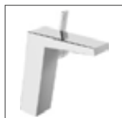
HANSALOFT one-hole single-lever basin mixer, DN 15 5769 2103 chrome for flat countertop washbasins, without pop-up waste, connection using copper pipes projection: 151 mm
