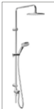
HANSAVIVA shower system water-bearing shower rail 4418 0200 chrome for connection with all exposed wall-mounted or all concealed mixers, HANSAVIVA handshower Ø 202 mm, HANSAVIVA hand shower, 100 mm, 3-spray
