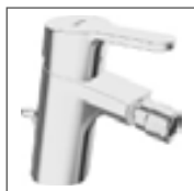
HANSAPRIMO one-hole single-lever mixer, DN 15 for bidet 4943 3203 chrome pop-up waste (metal), connection with flexible pressure hoses projection: 107 mm
