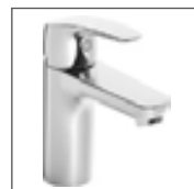
HANSA PINTO XL one-hole single-lever basin mixer, DN 15 4502 2283 chrome without pop-up waste, connection with flexible pressure hoses, HANSA 3S-Installation projection: 115 mm
