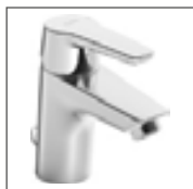
HANSAPOLO one-hole single-lever basin mixer, DN 15 5141 2293 chrome without pop-up waste, weighted chain, connection with flexible pressure hoses projection: 103 mm
