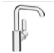
HANSAPRIMO one-hole single-lever basin mixer, DN 15 4955 2203 chrome without pop-up waste, connection with flexible pressure hoses projection: 142 mm
