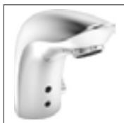
HANSAELECTRA electronic basin faucet, DN 15 battery-operated 6441 2210 chrome sensory operation (infrared), without pop-up waste projection: 96 mm
