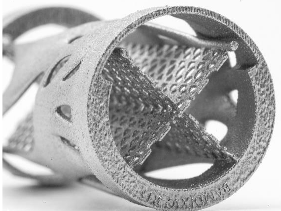
Figure 2: Redesign of a C-flex type pivot with interlocked crossed flexure blades
