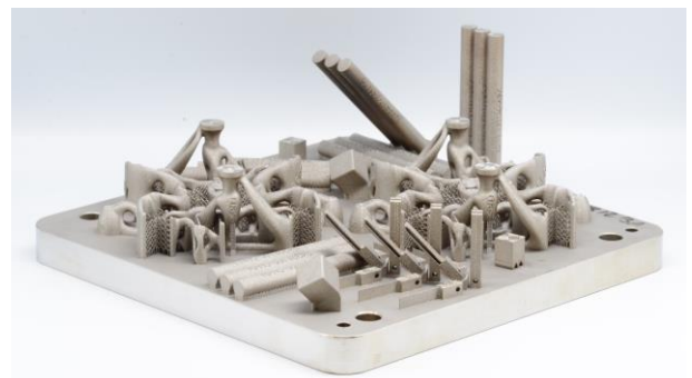
Figure 4: Build plate with two mechanisms and the batch samples
