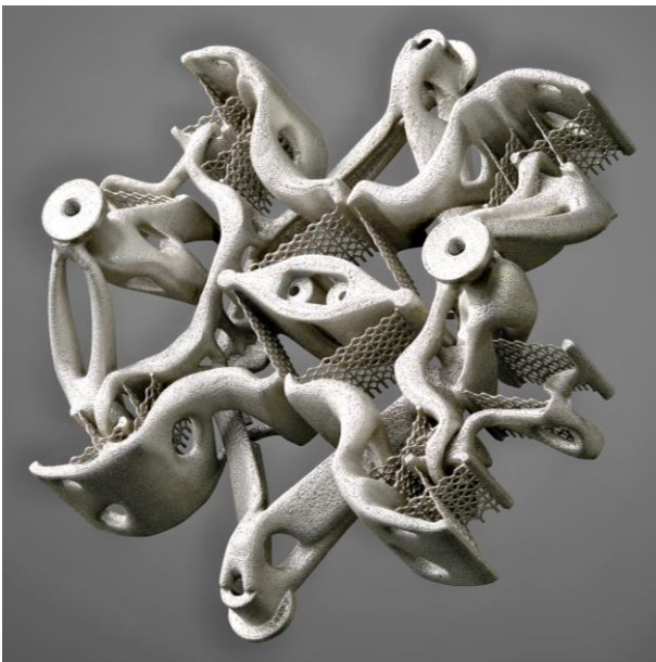
Figure 1: Compliant Rotation Reduction Mechanism (CRRM) built by Additive Manufacturing
