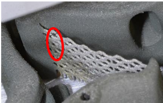
Figure 14: Damage of EBM1 following vibration test
