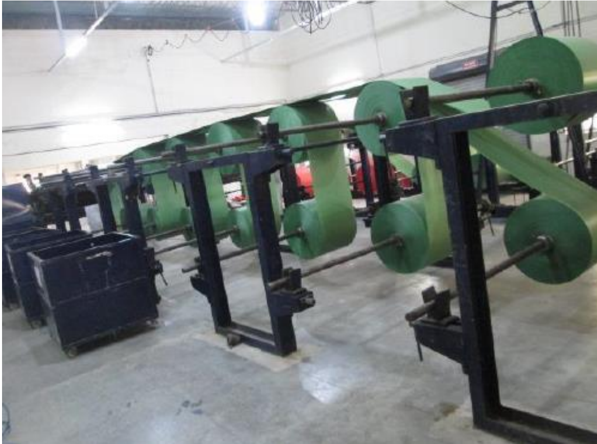
Sheet Cutting Machine – 200,000 cuts / DAY 3 machines
