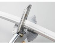
Use professional scissors to cut vertically at the cutting mark
