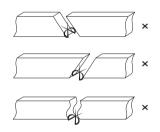
Please don't be feel free to cut and cut into an oblique angle or cambered section.
