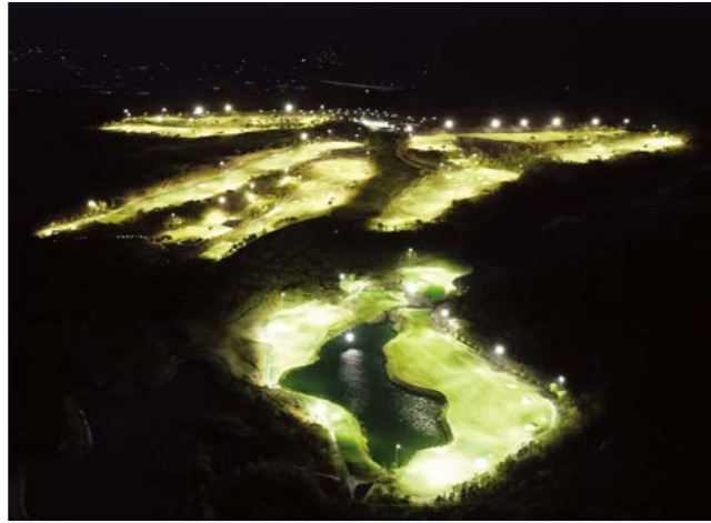
Ocean Hills Yeongcheon C.C. Light Level : 200-150-350LUX Fixture : LED 1200W (Q'ty:209) Pole : 15m, 18m (Q'ty:48)
