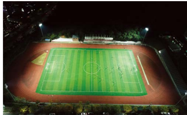
Gimpo Salter auxiliary soccer field Light Level : 400LUX Fixture : LED 1200W (Q'ty:48) Pole : 20m (Q'ty:4)
