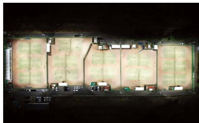
Gwangmyeong City Tennis Court Light Level : 500LUX Fixture : LED 1000W (Q'ty:60) Pole : 15m (Q'ty:12)
