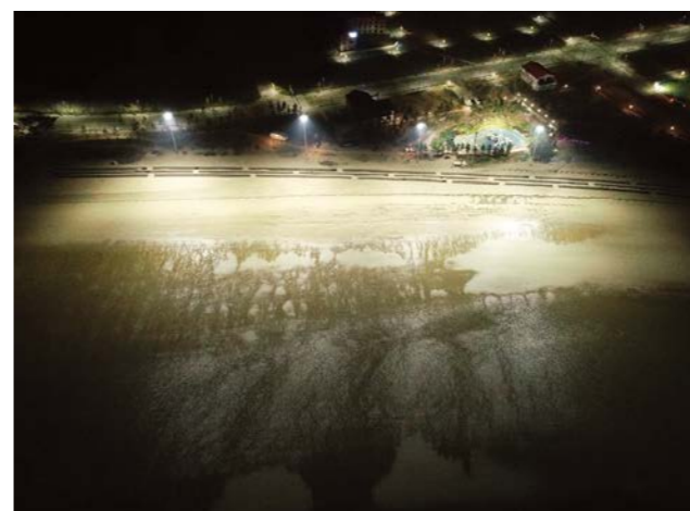
Byeonsan Beach Light Level : 60LUX Fixture : LED 1200W (Q'ty:22) Pole : 24m (Q'ty:4)
