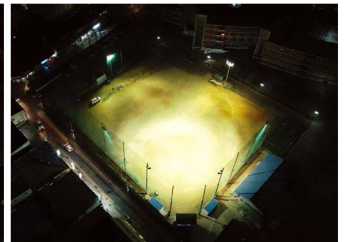
Gunsan Sinpung Elementary School Light Level : infield 300LUX Fixture : LED 1200W (Q'ty:14) Mounting Height: 18m
