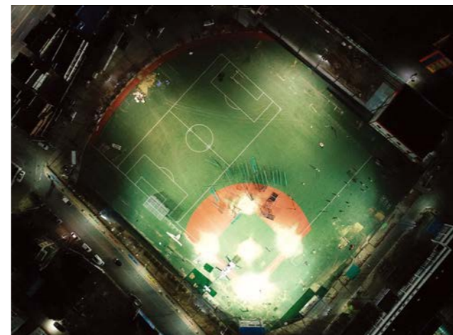
Gunsan Commercial High School Baseball Light Level : infield 250LUX Fixture : LED 1200W (Q'ty:10) Mounting Height: 20m
