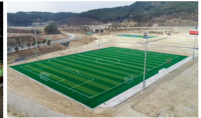
Seogunsan Soccer Field Light Level : 350LUX Fixture : LED 1200W (Q'ty:32) Pole : 24m (Q'ty:4)
