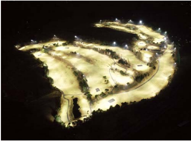
Gimje Anesville C.C. Light Level : 200-150-350LUX Fixture : LED 1200W (Q'ty:288) Pole : 15m, 18m
