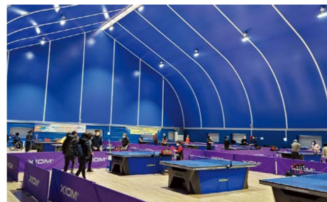
Gimpo Salteo Sports Park gym (table tennis) Light Level : 600LUX Fixture : LED 200W (Q'ty:24) Mounting Height : 10~12m
