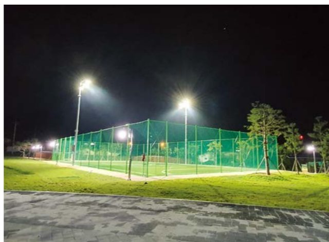
Gochang Sangha Sports Facility Futsal Field Light Level : 300LUX Fixture : LED 600W (Q'ty:8) Pole : 15m (Q'ty:2)
