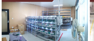
aging test room
