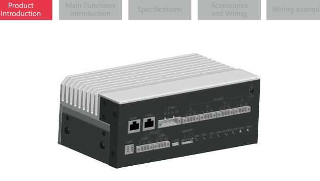
xPRO6 is an industrial-grade central control host that can be applied to smart buildings, smart factories, smart education, smart transportation and other scenarios, and is installed using DIN rails. This host system can customize the integrated management and control of different brands and models of products supporting RS485, RS232 and LAN control. Make the IoT access operation of equipment more humane, more environmentally friendly and more efficient.
