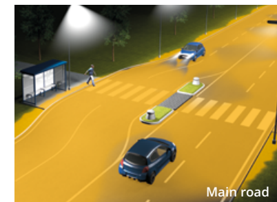
AREDO Design with O3, O7 or O13 lens system, optimized for M classes, with excellent edge illuminance and a pole height - and long pole spacing ratio of up to 1:6
