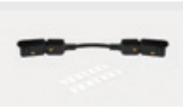
I-shaped electrical connector (recessed type) Model: TLS-M265 Size: L70×W11.5×H2.1mm(Splicing bar) L78×W19×H17mm(Power feeder) Applicable model: TLS-MR2X0A TLS-MR2X0B TLS-MR2X0C
