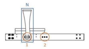
8. If necessary, change the inclination of the light fitting on the console by regulating the light fitting bracket (from -20° to +20°).
