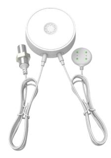
Aqua-Scope offers an alternative solution based on water sound. The microphone is mounted on a water pipe and 'listens' to the water. It detects all water activities in the whole system thanks to the water's excellent sound conduction. This water monitor fulfills two functions: On the one hand, it determines the water consumption in the house or apartment, and on the other hand, it detects different types of water leaks.
