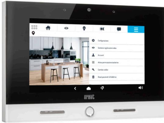
The new 7" touch keypad is the core of the Urmet 1068 system: from a single control point you can manage **intrusion alarms**, **video surveillance** devices, **video door phone systems** and **building automation**, also through special scenarios.
