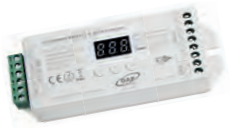
DMX-DECODER Enables RGB|RGBW|RGB CCT to be DMX compatible Supply voltage: DC 5V | 12V | 24V RGB output: 3 channel RGBW output: 4 channel Static power consumption: <1W Output: 5v:<80W, 12V:<192W, 24V:<384W
