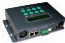
T-DMX512 RGB Master Controller Hand held remote Multiple lighting functions Various colour changing programs Programs can be varied in speed Compatible with DMX 512 sources Dimension: 163 x 108 x 40
