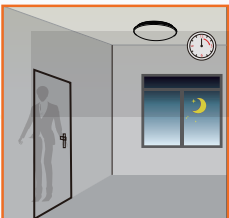
The light automatically turn off 60 seconds after human leave.
