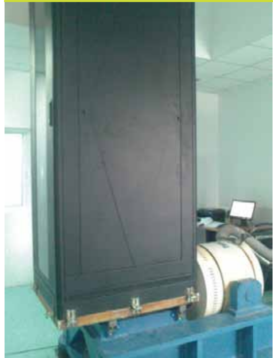
Dynamic load, vibration and mechanical impact tests (DL4)
