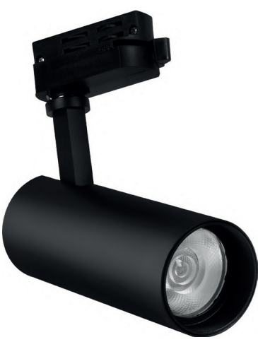
Shopline BD30-51401 15W 3000K 1180lm Black 220-240V CRI>80 IP20 Aluminium 4-Wires
