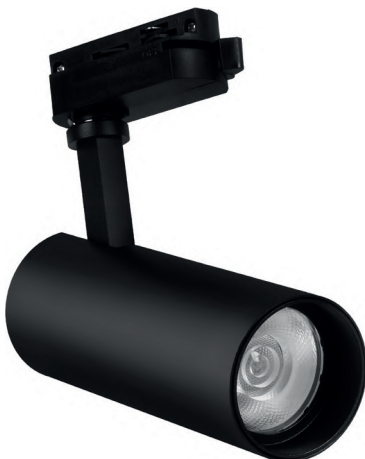
Shopline BD30-01401 15W 3000K 1180lm Black 220-240V CRI>80 IP20 Aluminium 2-Wires
