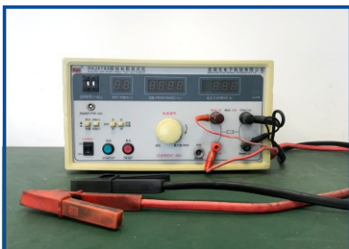
Ground Resistance Test
