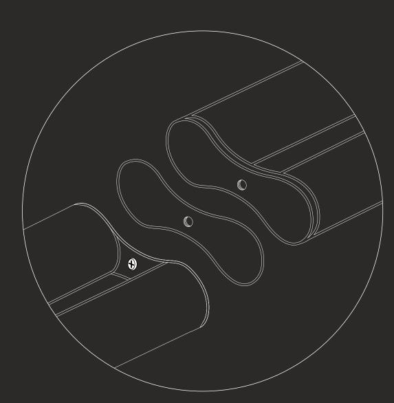
2 Trigon lamps are connected with custom CNC cut to shape connector. It may be applied onto any arm of the fixture, enabling the modular extension of the system into chosen direction by adding consecutive Trigon lamps.
