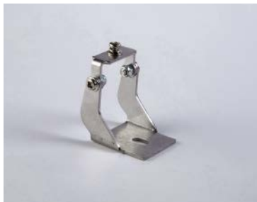
Angle adjustable Bracket Dimension(LxWxH): 25.5*28.5*38.5mm Material: Stainless steel 201
