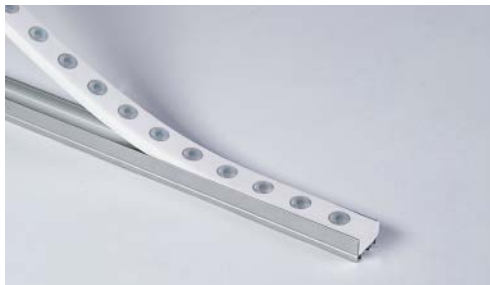
Aluminum Profile (No baffle) Dimension(LxWxH): 1000 x23.6*17.6mm Material: Aluminum 6063
