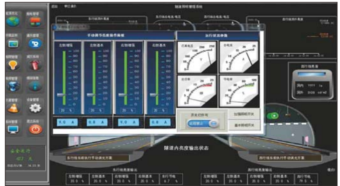
▲ 在特定情况可手动控制灯具的亮度 The luminance of the lamp can be manually controlled under certain circumstances
