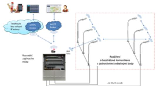
Pic. The concept of wireless communication designed for public lighting switching point communicating with the superior control (dispatch) room, communication with service personnel and communication with each slave lamp. Our new Foxtrot 2 serves as the communication and control centre. Other sensors may also be connected via the network using the 868 MHz band, which allows the user to expand the Internet of Things (IoT) even further.
