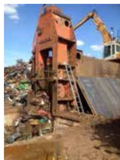
HENSCHEL hydraulic crusher with a pressure of 850 tons is used to do so. Because there were daily breakdowns the crusher control system required a modernization. Frequent outages often required very complex servicing interventions resulting in a significantly reduced productivity.
