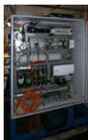
Foxtrot CP1005, MR0161, SX1165, 4x IB1301, 3x OS1401, Easy View touch screen. Disk RPM control : 2 analogue outputs - 3 servo drive, CAN, RS232 - used to enter key identification information for embossing, Ethernet connection used for PLC programming, touch screen, local network - master key entry, printer - prints combinations of different depths of key notches, as well as the type markings and the specification of the security level on plastic security cards.
