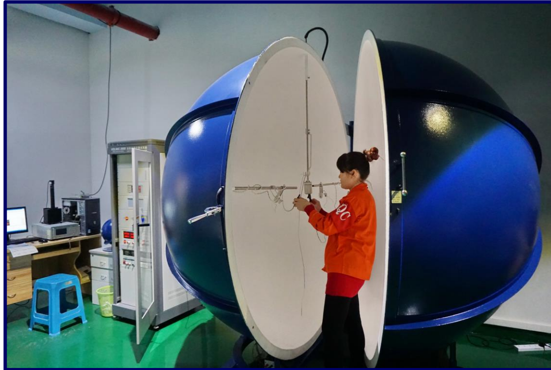
Light Source Analyzer with Integration Spheres
