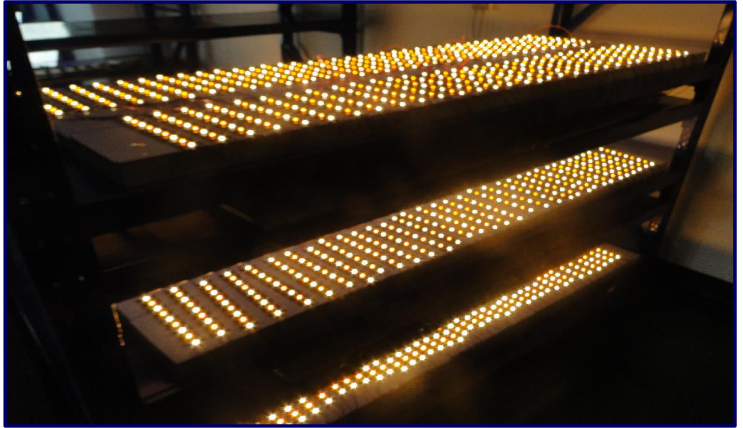
High power module burn-in with heat sink
