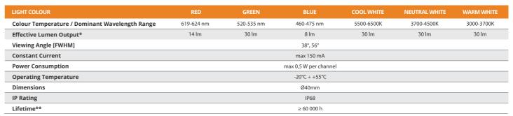
\* Source performance in real-life conditions at Ta=25°C; includes optical losses; the tolerance of source lumen output is 10%.
