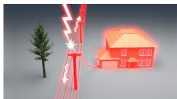
3. Strike on overhead lines
