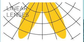
Linear lens profiles are used to create special lighting patterns with highest efficiency and protect the light source at the same time.
