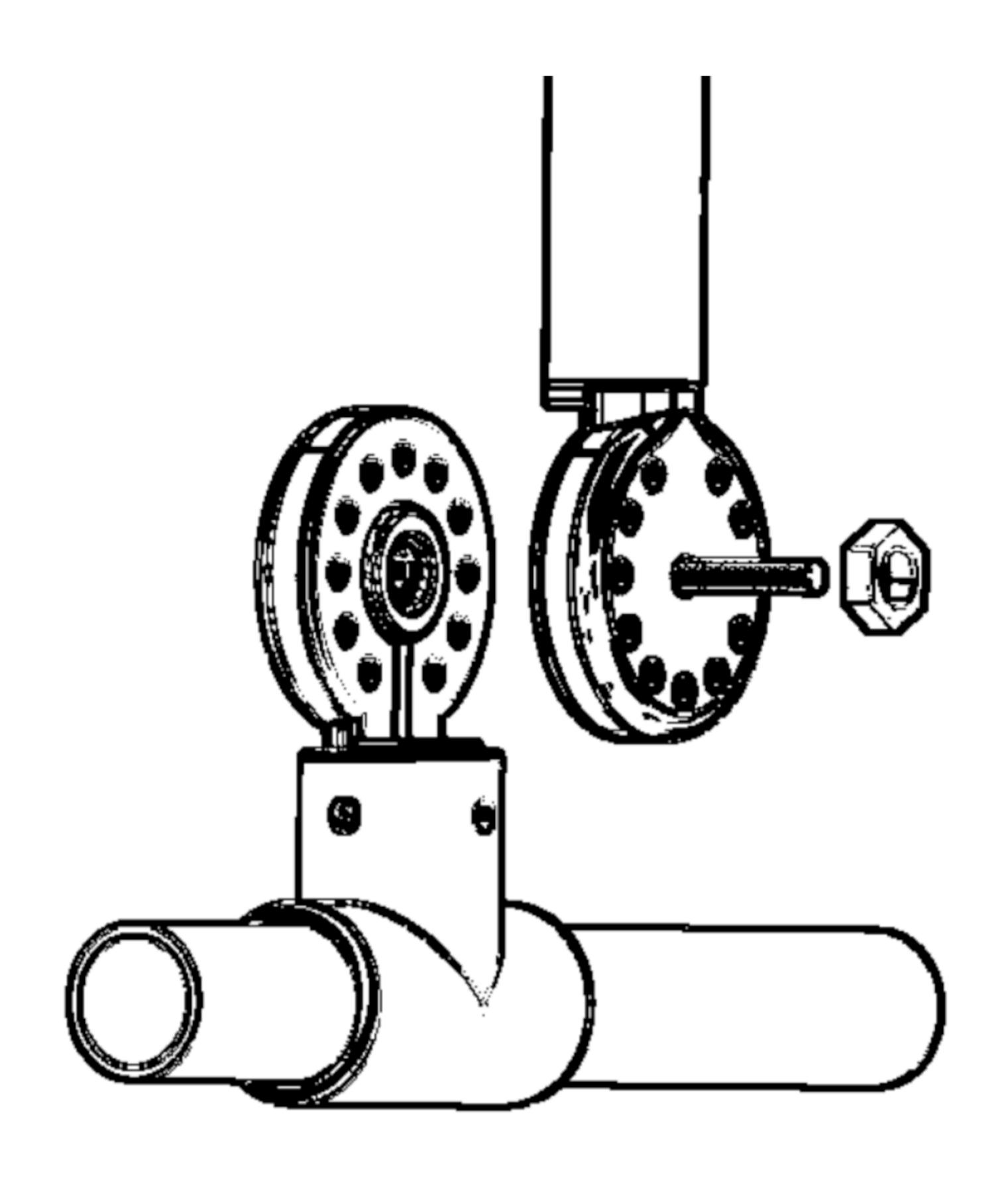
The tubes and light elements can be interconnected with a current carrying hinge. Customised compositions can be made upon request.
