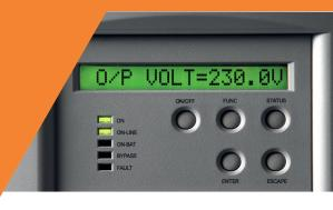
UPS systems of the type JOVYTEC P are available with power ranges of 700 VA up to 3 kVA. Due to their online double converter technology these UPS systems meet the requirements of the highest protection class VFI-SS-111. During start-up a diagnostic test system is activated verifying the status of the UPS system and the battery. The power related fan control system protects the system against overheating and ensures a long battery life.
