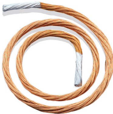
Litz Wire Size: 0.125mm Configuration: 5x3x28
