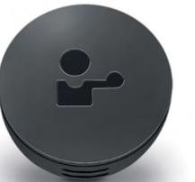
TraqFreq is attached to an instrument and integrates an accelerometer, and temperature and humidity sensors, enabling it to monitor both climate conditions and playing time. Monitoring the instrument can assist in extending its lifespan. And by measuring playing time, TraqFreq can also determine the lifespan of instrument consumables
