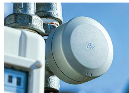
The sensors integrate Nordic's [nRF9160](#) SiP to provide LTE-M connectivity to relay data to the cellular network and in turn to Braveridge's BraveGATE Cloud Service where management can review the data.
