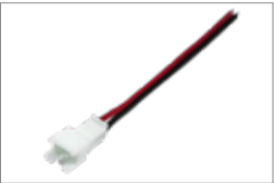
SM-2A female connector, 2 cores, UL2468 20AWG L=80/2mm
