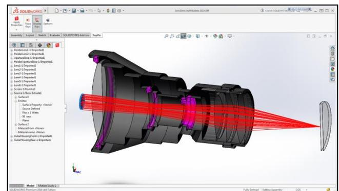
**Figure 5:** Use cut-away views to ascertain ray propagation and beam profile through assemblies
