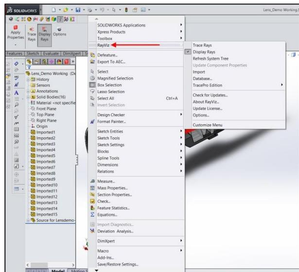
**Figure 2: RayViz Menu added to SOLIDWORKS**
