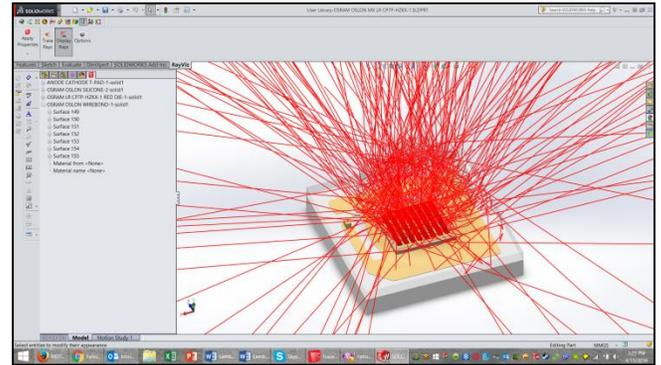
**Figure 3:** Insert an Existing Part to an Assembly add source definition and raytrace
