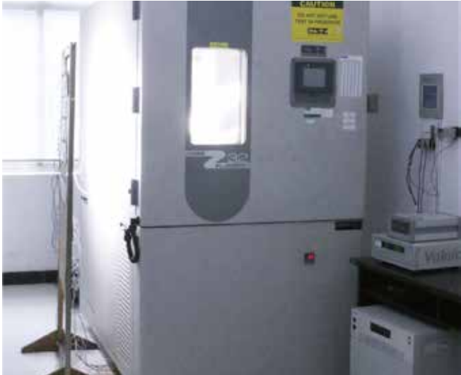
Temperature and humidity cycle test box
