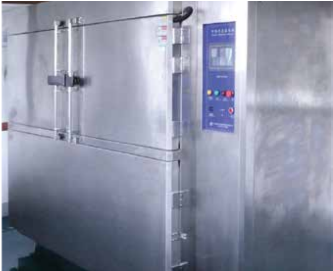
MAX.1.5m cold and hot impact test box
