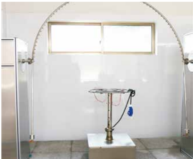
IP testing chamber
