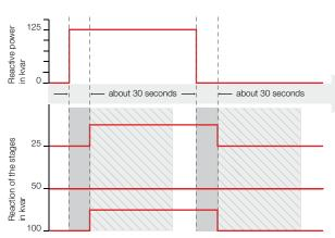
Switching times with contactors
