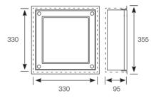
Flush mounting dimensions: 330 mm x 330 mm x 95 mm
