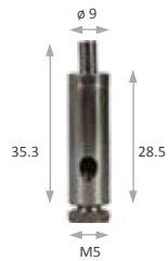
CODE : GPCB-219H WIRE : \phi 1.2-1.5mm
