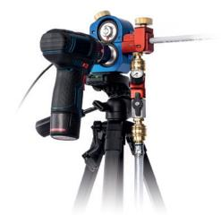
The X-Blow Micro consists of a feeding device, a separate blowing chamber for 2-3 mm or 4-5 mm cables, a compressed air unit with display and air-pressure regulation.
