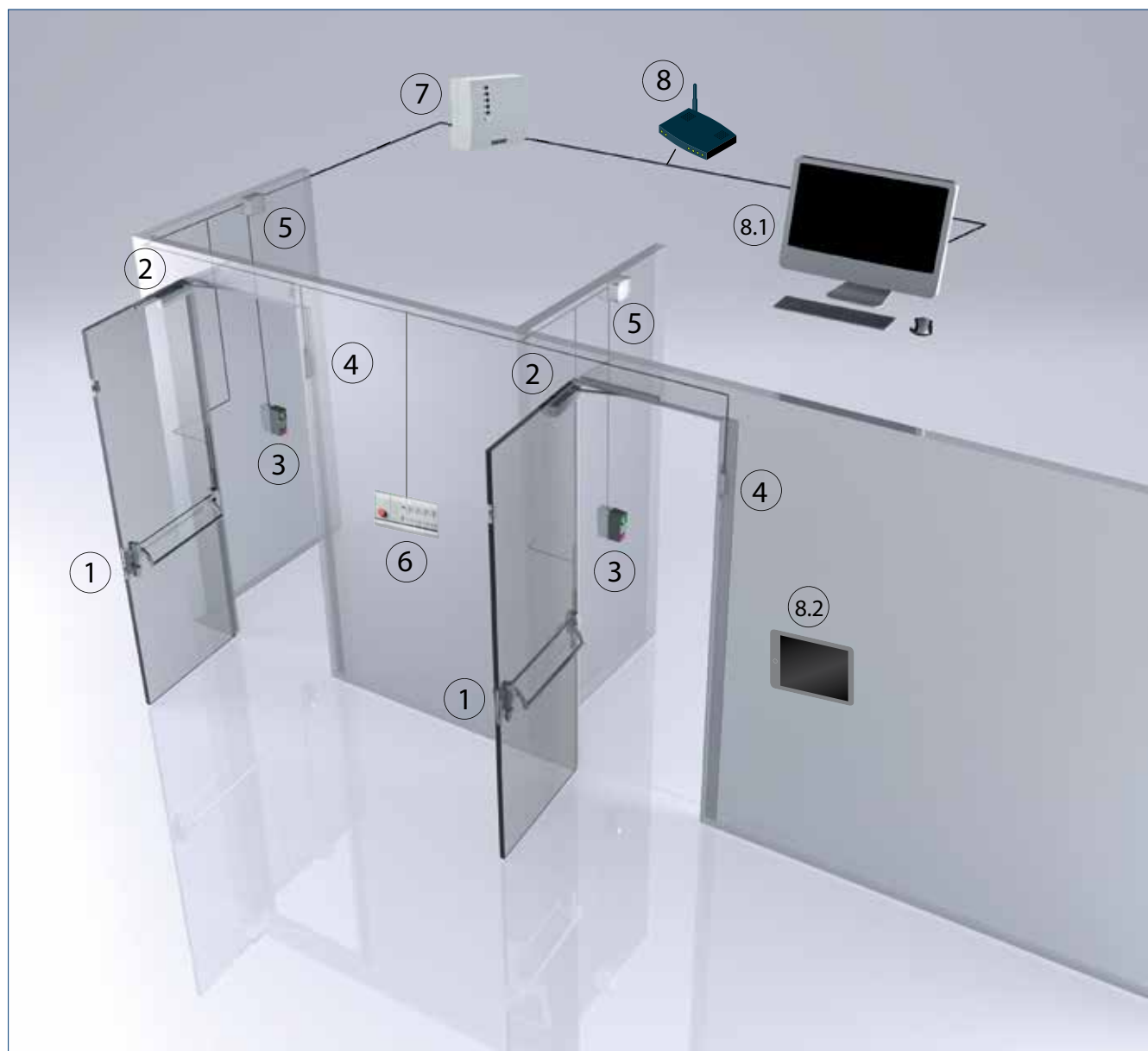
1 = IQ lock EL motor lock | 2 = TS 4000/TS 5000 door closer | 3 = TZ 320 door control unit | 4 = FTV 320 escape door lock | 5 = MST 210 motor lock control | 6 = TE 220 control panel | 7 = GEZE Cockpit | 8 = router (optional) | 8.1 = GEZE Cockpit VISU on desktop PC | 8.2 = GEZE Cockpit VISU on touch screen (optional)
