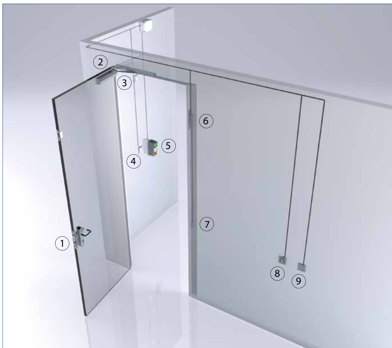
1 = panic lock with exchange function "E" on site | 2 = TS 4000/TS 5000 door closer | 3 = push button at 1.80 m height | 4 = switch to activate or deactivate the exterior push button | 5 = TZ 320 SN door control unit, surface-mounted/flush-mounted | 6 = FTV 320 escape door lock | 7 = A5000--B electric strike | 8 = key switch | 9 = push button outside
