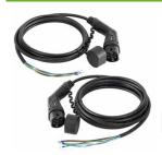
Charging cable – AC charging cable with Type 2 charging connector in accordance with IEC 62196 and open cable ends, with cap, cable construction  $5 \times 2.5 \text{ mm}^2 + 1 \times 0.5 \text{ mm}^2$ , IP54 (with cap), charging power up to max. 11 kW (3-phase), charging current up to max. 16 A, for installation on a Spelsberg Wallbox
