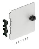
Inner door made of insulating material for installation in GEOS cabinets, incl. fixing material and rotary twist lock with key, 3mm double bit, for individual use, e.g. for installation of displays, command and signalling devices, material thickness: 4 mm
