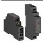
Mains supply unit for assembly on NS35 standard rail. Input voltage 85V to 264 V AC, output voltage 21.6 V -29 V DC. Output max. 15.2 W.
