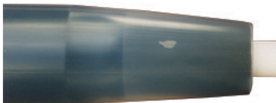
Fig. 3: Disappearance of an air bubble in the gap between the sleeve insulating body and the FSE.
