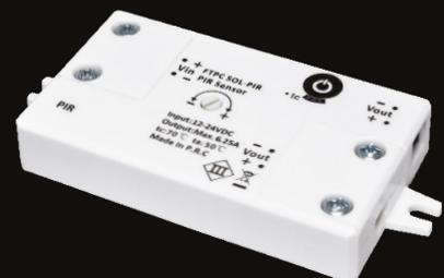
**FTPC-SOL-PIR+S103** - Output side Human-body detection PIR sensor (Low Voltage), detection range < 2,5 m / 80 degree / 10s-3min + probe.
