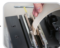
Heated jaws activate the glue during the quick installation process
