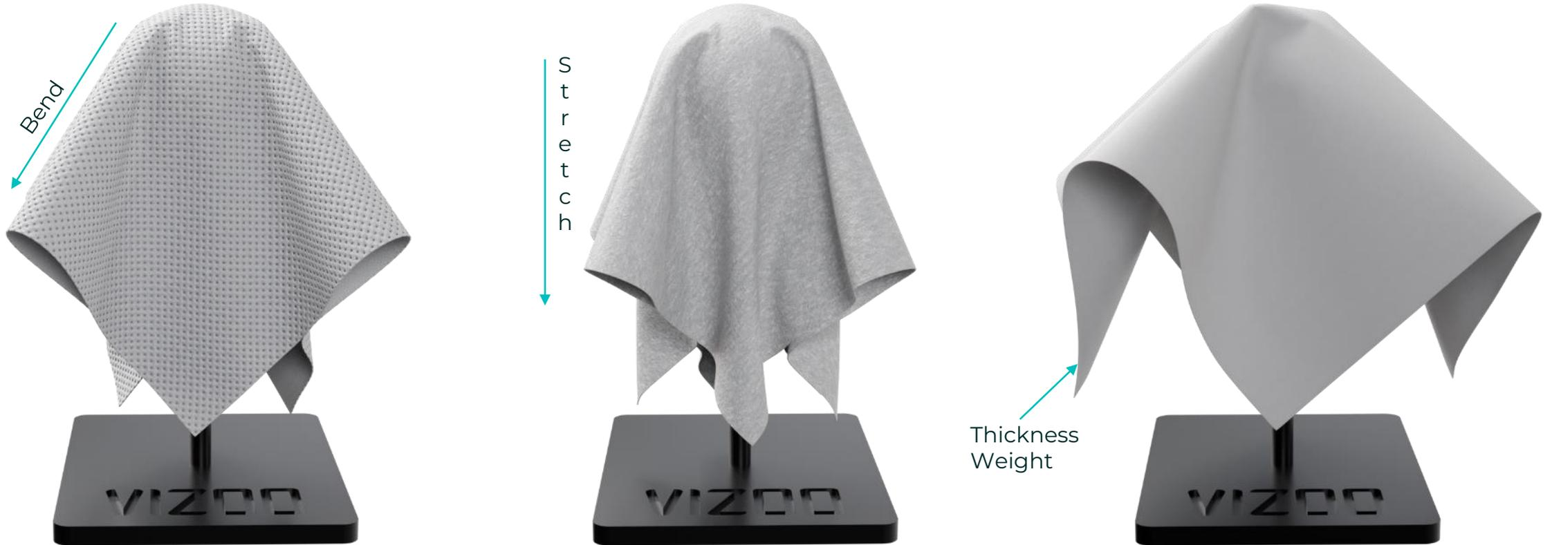
The drape of a material is dependent on parameters like bend, stretch, weight, and thickness.
