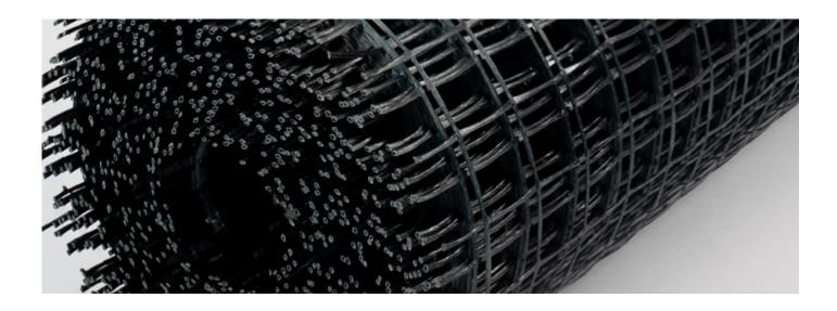
This specific mesh is intended to reinforce floor screeds, cement, and lime plasters. Big mesh sizes of 40×40 mm facilitate mesh sinking in concrete. The standard technique of strengthening screed floors with steel wire trusses is challenging to install and costly to transport. Compact size and light weight enable rapid and straightforward installation and prevent the high costs of transporting big objects.
