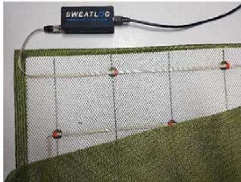
Fig. 6.7. SWEATLOG logger and sensor array (mat) with up to 60 HIH8xxx sensors at one I2C ribbon (4 wires).
