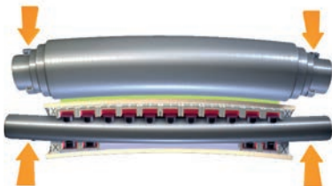
Roll retraction at full fabric width
