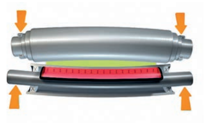
Increased line force at the edges
