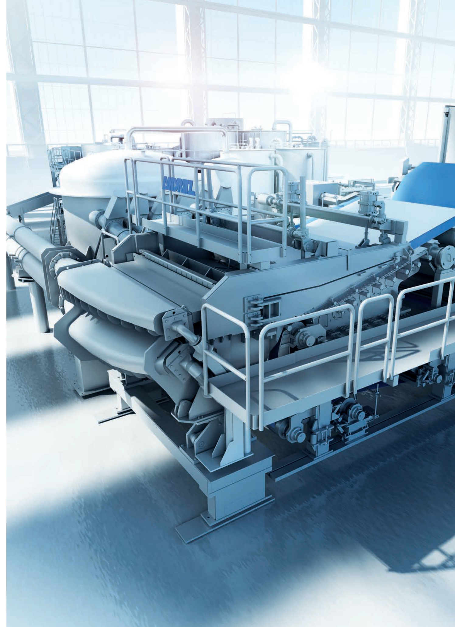
neXformer eXcelle forming unit with multi-layer headbox
