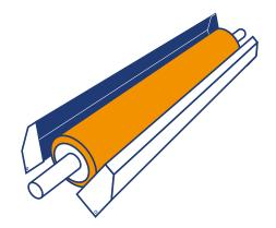
When activated lateral cover open, cleaning cylinder move up and push the web to the back roller on top. Running of web drives both rollers avoiding issues on speed synchronization.
