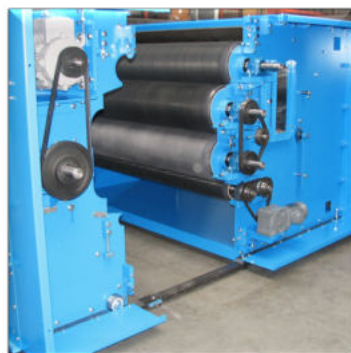
Machine opening for easy cleaning and maintenance.
